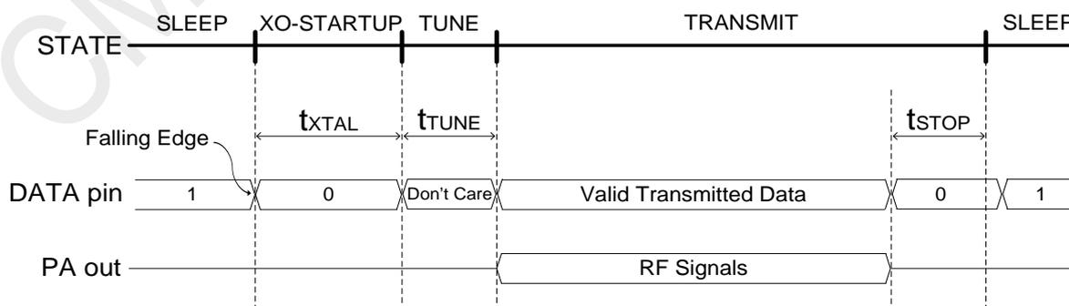
Figure 9. Transmission Enabled by DATA Pin Falling Edge
